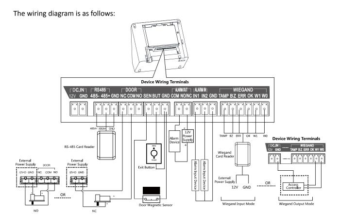
You can also connect the terminal with the seucure door control unit. The wiring diagram is as follows:
